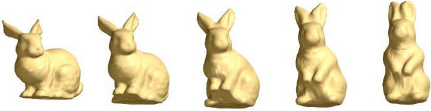
Fig. 4. Mesh morphing of two bunny models based on Poisson shape interpolation. Instead of absolute vertex positions, gradient fields (or Laplace coordinates) are interpolated as D_t = (1 - t) D_0 + t D_1 , and the vertex positions are derived by solving the Poisson system \Delta X_t = D_t (Image courtesy of Xu et al.)
